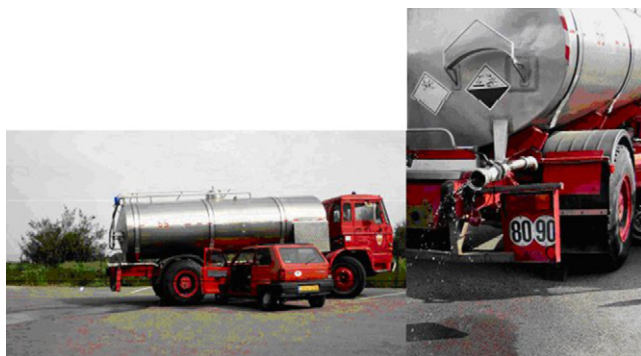
Fig. 8. Scenario representing the collision between the tank truck and the light vehicle with a detail of the chlorine leak.
